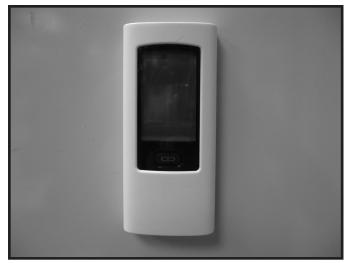
Figure 12.8 Mounting Remote Control Housing
